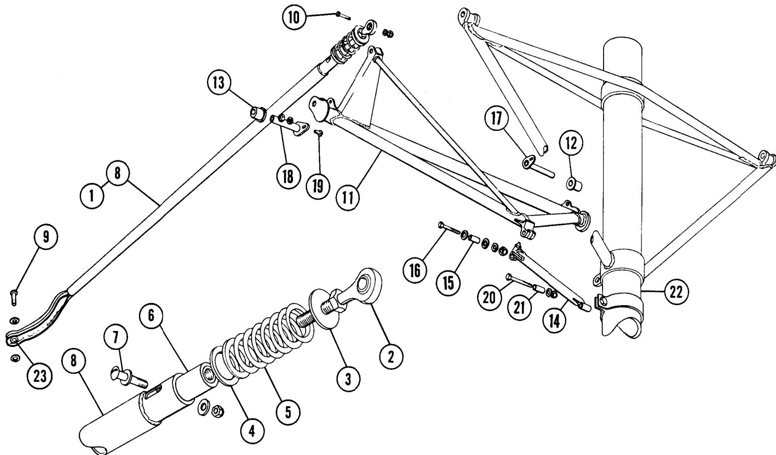
Figure 42. Landing Gear Retract Mechanism
